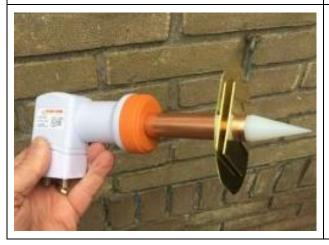
• The dish mount is placed just behind the Patch reflector, not on the LNB!
