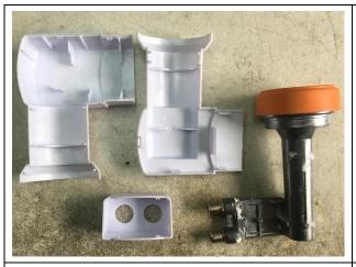
• Remove the plastic covers starting with the cap at the connector side.
