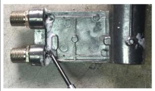
Remove all sealant with a small screwdriver.
